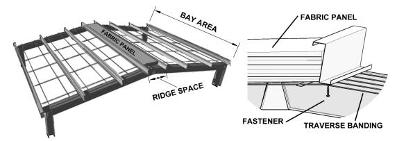
3. Pull one edge of the fabric under the purlins and on top of the banding while making sure the finished side (usually white) faces down toward the building's interior. Complete one half of the bay at a time. For easiest deployment, it is recommended that two (2) workers at each edge of the fabric bundle place a 1'0" upward and inward folded tab on both edges nearest the rafters as the fabric is deployed so that the edges won't hang up at the purlin/rafter connection point.
