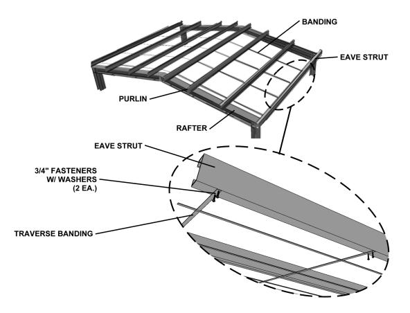
4. Pull each band hand-tight towards the ridge purlins while weaving above every 7<sup>th</sup> or 8<sup>th</sup> longitudinal band and above the bands in the ridge space. Fasten to the ridge purlins and far eave strut using one (1) of the <sup>3</sup>/<sub>4</sub>" TEK 3 fasteners with washers provided. **Do not fasten into purlins at this point.**
