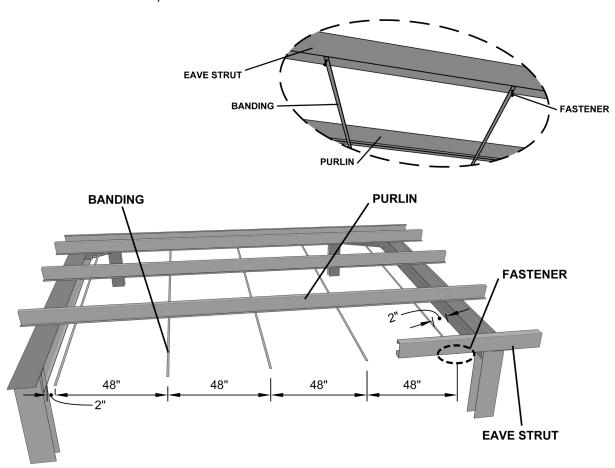
4. For additional fabric support, install two (2) longitudinal bands within the ridge space of a double slope building and pull each traverse band tight towards the ridge, over the ridge bands and down to the far eave. Fasten traverse banding to the ridge purlins and far eave strut using one (1) of the 3/4" TEK 3 fasteners with washers provided. Do not fasten into purlins at this point.
