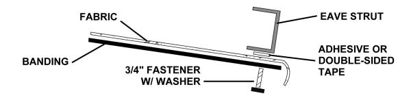
4. Repeat for each band and complete the fabric installation by pulling the fabric in opposing directions towards the rafters, working out wrinkles and securing traverse banding at each purlin intersection with a ¾" TEK 3 fastener with washer. Do not fasten the 2" rafter band at this point, as it will be secured after the insulation has been installed.
