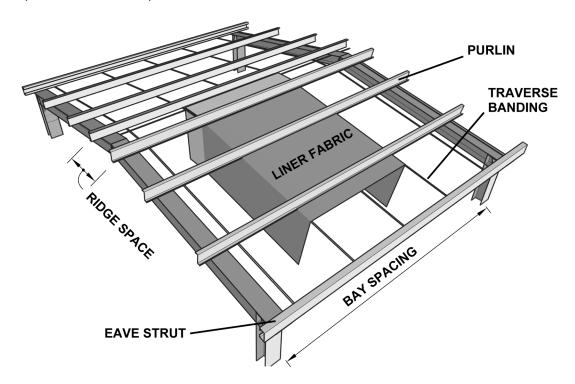
2. Pull the leading edge of fabric toward the eave making sure the finished side (usually white) is facing downward towards the building interior. Once the fabric is square to the eave and rafters, begin securing the fabric and banding to the near eave purlin using the ¾" TEK 3 fasteners with washers. Then, work the fabric back towards the far eave purlin and secure in the same manner.
